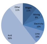
The other 5 major areas that comprise mine site cash costs are evenly distributed between; Lime - used for neutralisation, Electricity - used for electrowinning the nickel cathode production, Mining – for both ore and waste movement, Wages – for all staff, and other mine site cash costs.
