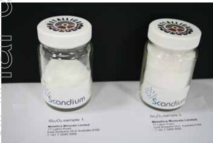
High purity scandium oxide produced in pilot testing by processing Metallica's material from SCONI, July 2012
