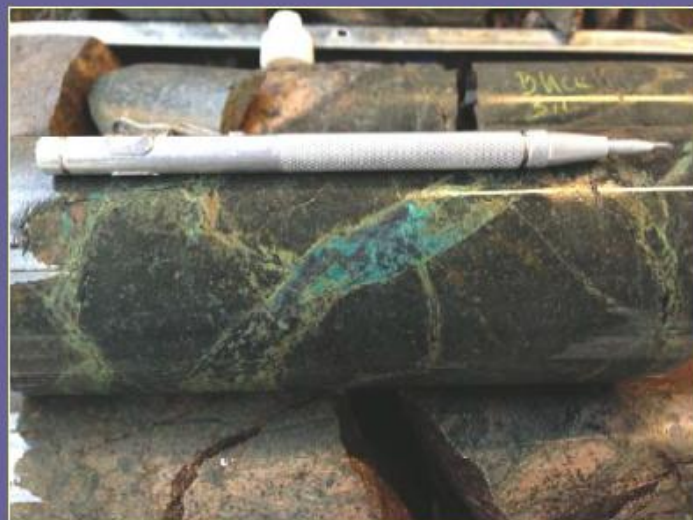
Photograph of mineralized breccia (Hole 2 at 61m)
