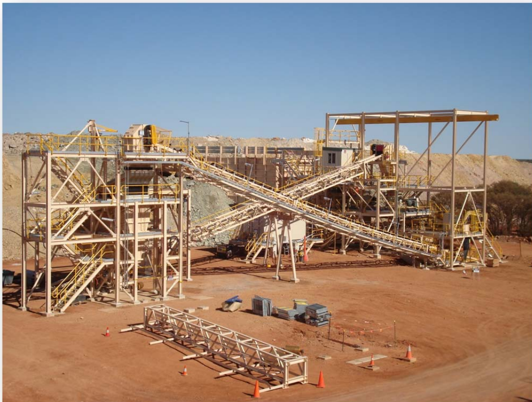
Figure 2. Crusher and screening buildings with ROM in background.
