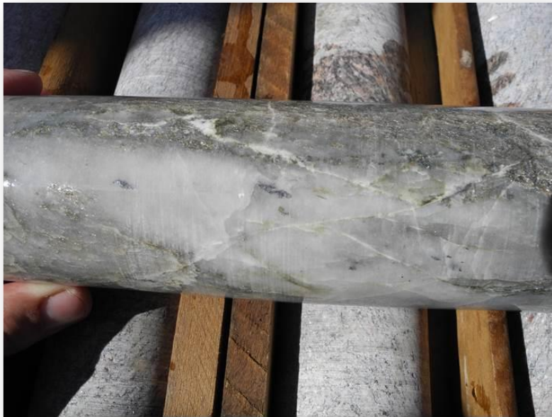
NCD004 mineralisation – 8 metres @ 15.33g/t gold
