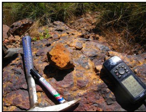
Iron Ore prospect: terrain and sampling; grades up to 63.7% Fe
