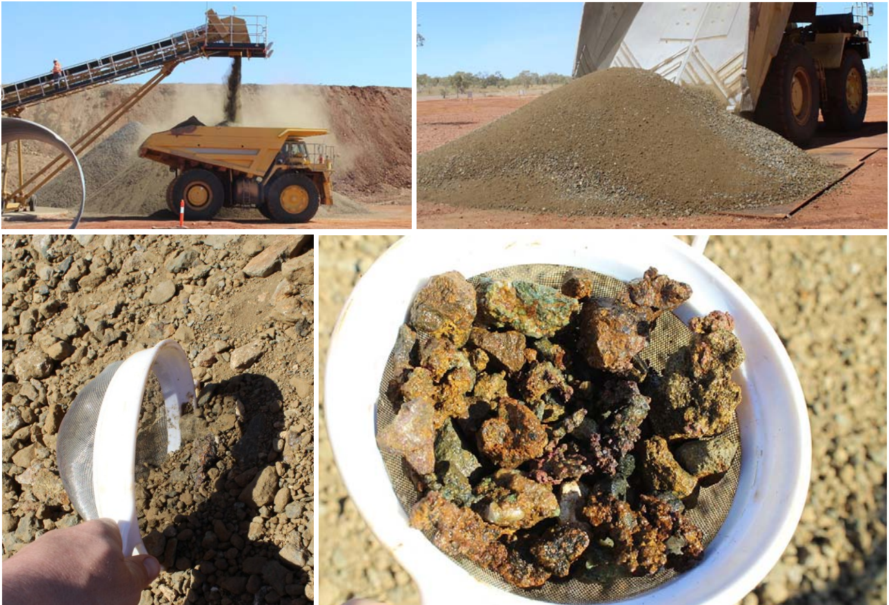
Figure 10: Commissioning activities at crushing circuit included processing high-grade native copper ore. Above example of randomly sampled ore cleaned with water, dominated by copper minerals native copper, malachite, cuprite and minor chalcocite. This sample visually estimated at 22-26% Cu.
