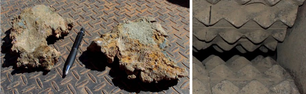
Figure 6: Samples of coarse native copper ripped and flattened by the first-stage roller - "teeth imprints" clearly visible on the left native copper sample.
