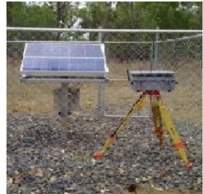
Figure 23: Solar powered DRX dust track real-time dust monitor.
