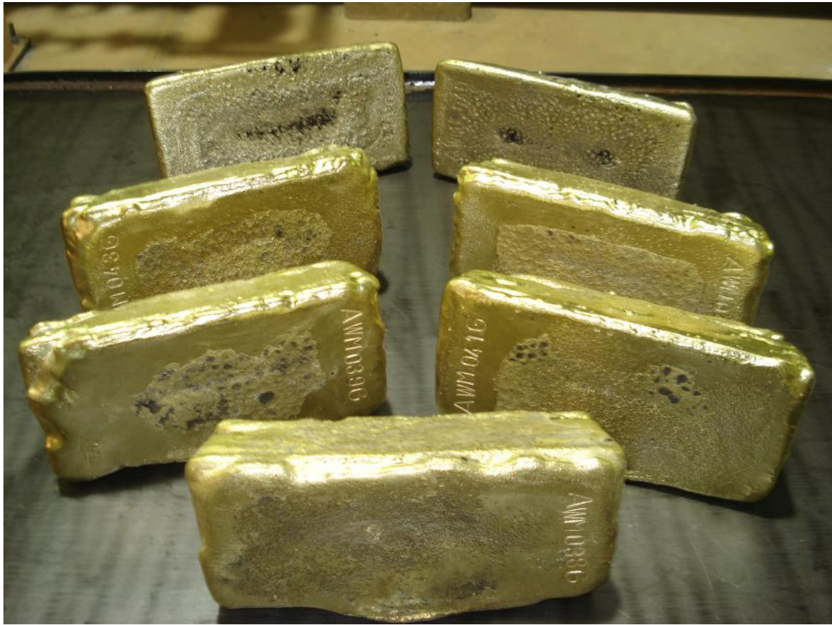
Figure 2. Gold production from the last week of September – a combined 89.26kg (approx. 2,870oz) of doré from the gravity and leach circuits.
