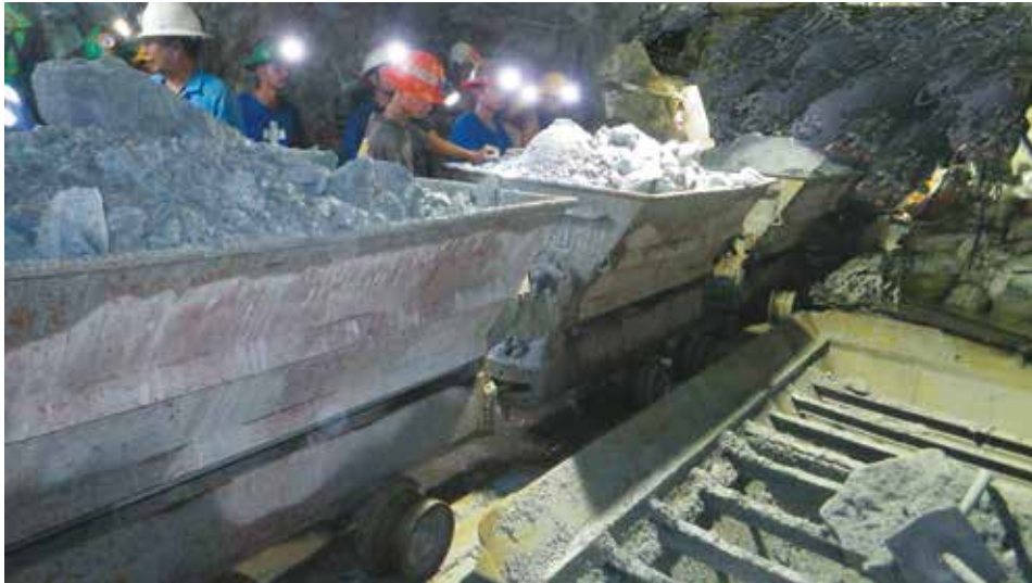
Photo 5: Loading ore into loading pocket 8L
