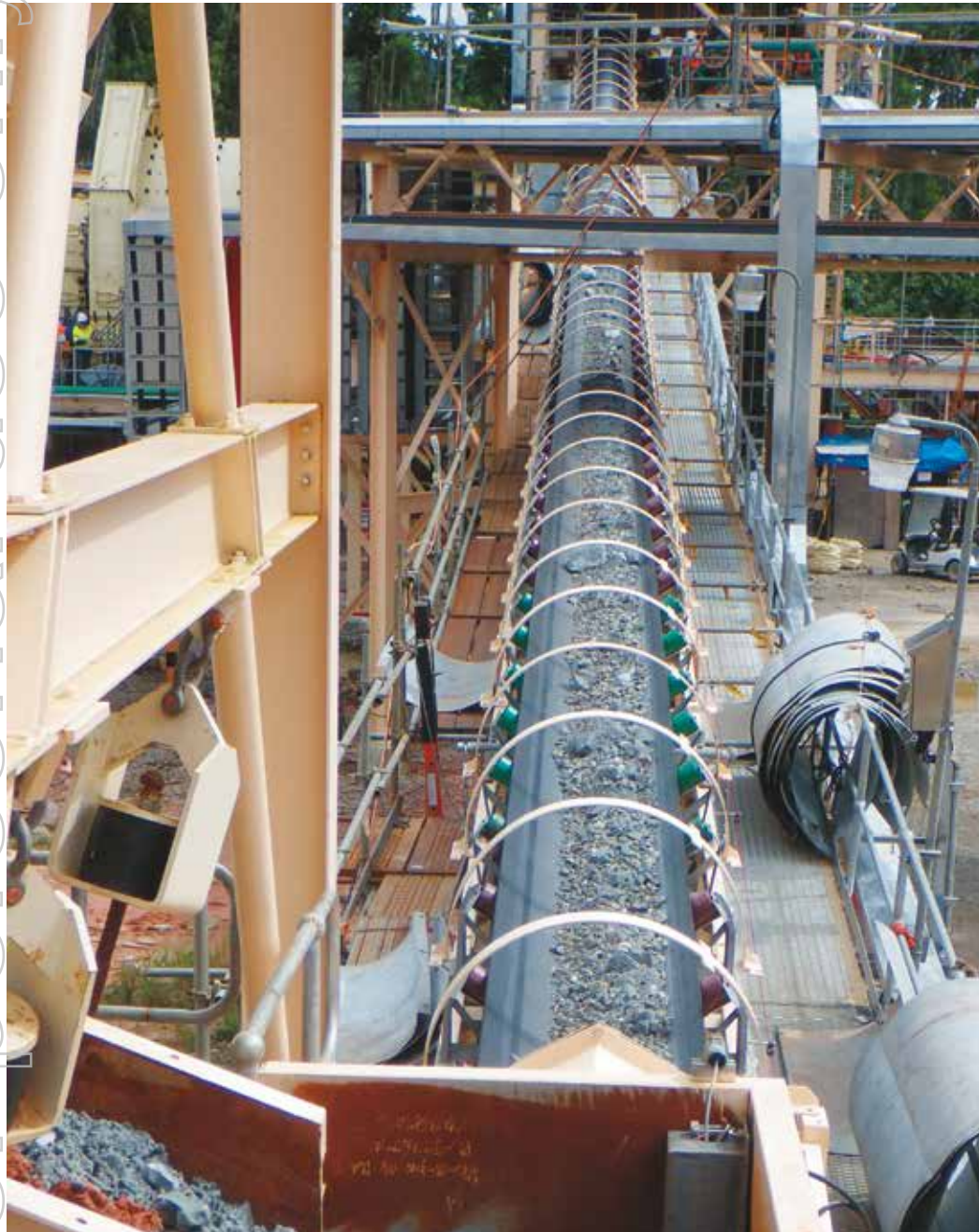
Photo 1: Crushed ore being loaded into Sag Mill
