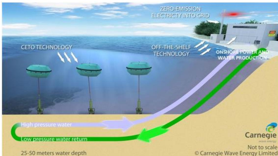
The CETO system is different from other wave energy devices because it operates under water and is anchored to the ocean floor. Several fully submerged buoys are tethered to seabed pump units. The buoys move with the motion of the passing waves and drive pumps. The pumps pressurise water which is delivered onshore via an underwater pipe.
