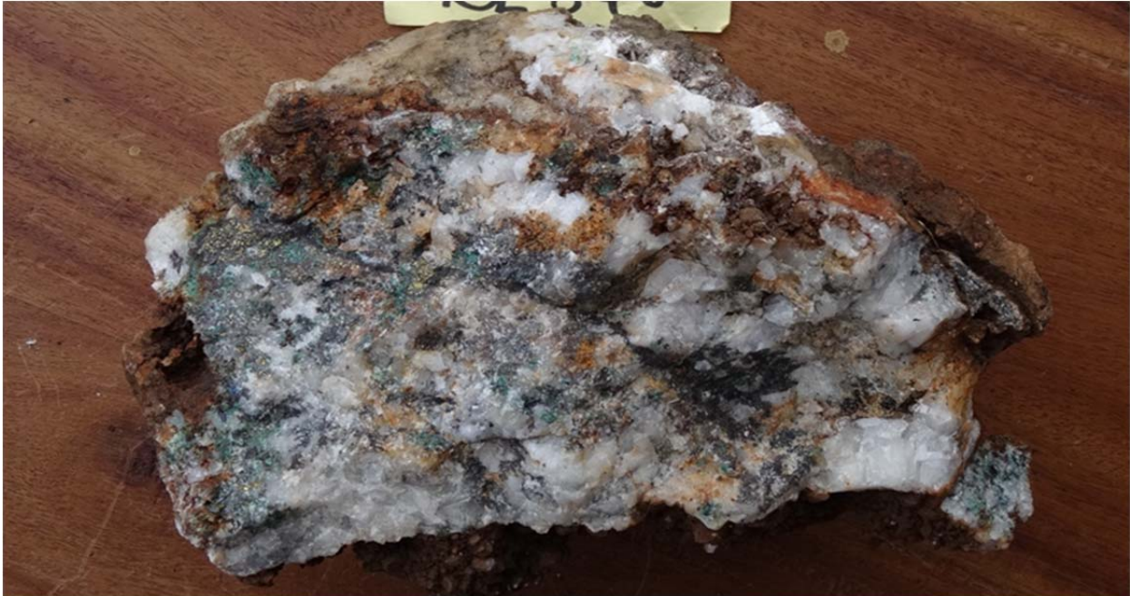
Figure 2: Sample E28-008. Vein quartz with calcite veinlets, pyrite, chalcocopyrite and copper oxides
