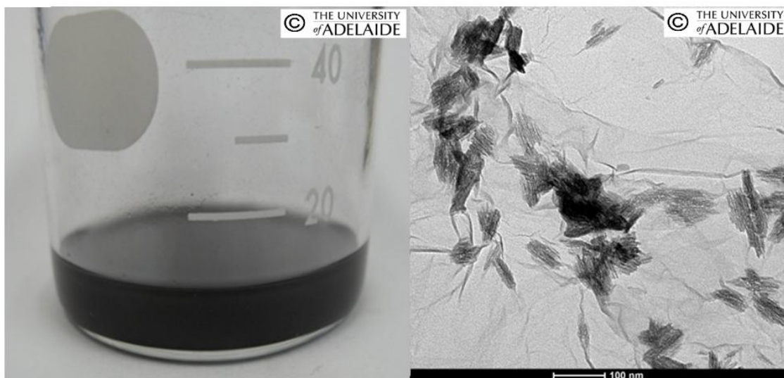
Plate 2. Prepared graphene nanosheets in solution from raw Archer Campona graphite. (Left is TEM image)
