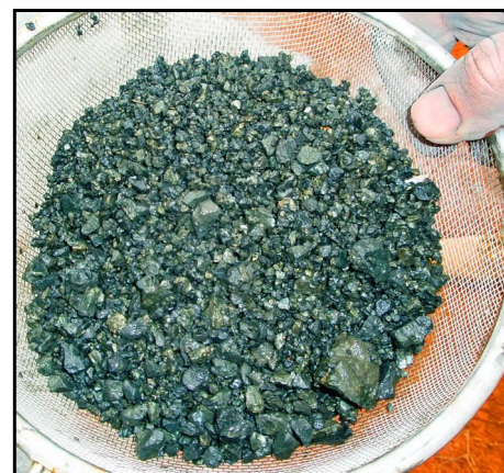
Manchego Phase 1 drilling: RC Drill Chips from MRC 040 (74-75m) showing sulphide mineralisation within gabbro-norite host
