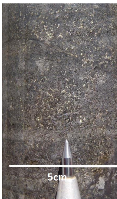
Figure 5b: Disseminated sulphide in drill hole PALDDH001 from 41.1m down hole.
