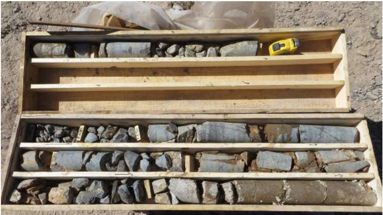
Figure 2: HQ diameter diamond core from the start of drill hole DHC-01 at Colupo (Dec 13).
