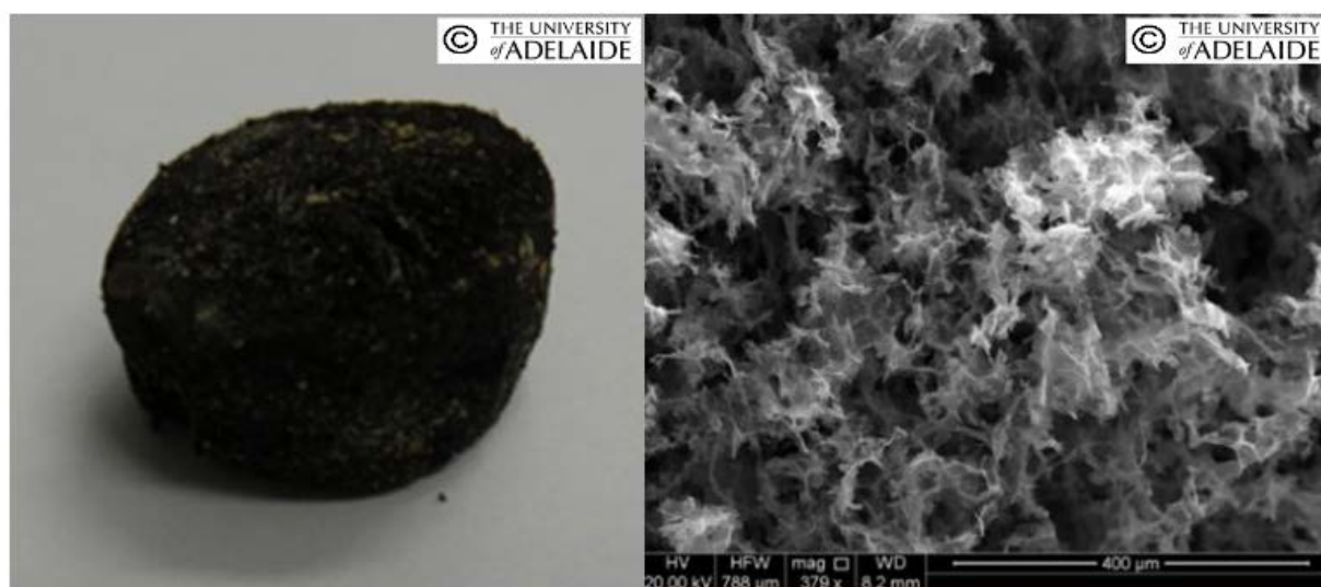
Plate 5. Prepared graphene aerogel filters for water and air purification from raw Campona graphite
