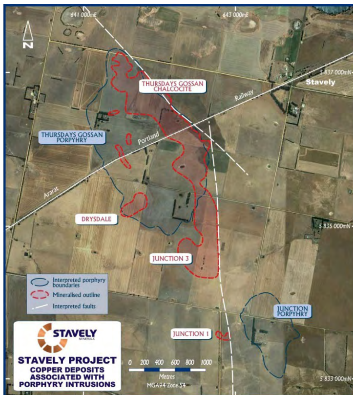
Figure 20. Prospect location map on air photo showing Ararat to Portland railway, chalcocite-enriched Mineral Resource (red outline), major NW and NNW structural controls (white dashed) and porphyry outlines (blue) as interpreted from gravity, magnetic and drilling data.
