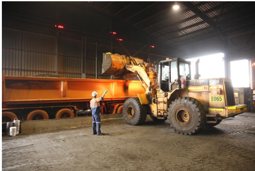
Loading nickel concentrate into half height containers
