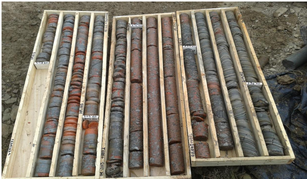
Figure 1: Photos of core in the field from DDH J13-08 showing potash mineralisation (red)
