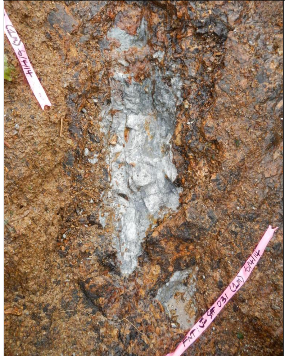
Photo 4. Sample J-031 from Trench 1, with 163.0 g/t gold in gravimetric analysis, but 38.0 g/t gold in 50 gram fire assay. This was the only significant 'anomaly' or difference between the 2 types of analyses.
