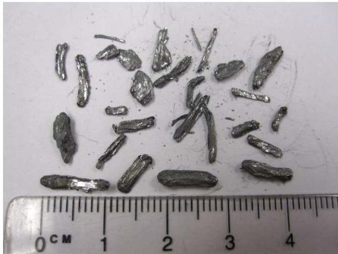
Plate 5. Flake aggregates from RC drill hole WG041 (98-99m). Scale bar in centimetres.
