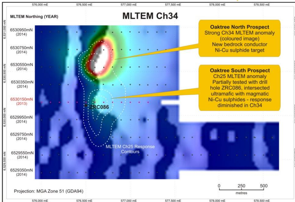
Figure 3. Oaktree Prospect (previously ZV10) showing MLTEM lines from 2013 & 2014, location of drill hole ZRC086 that intersected magmatic nickel-copper sulphides, MLTEM Z component Channel 25 (18msec) contours, over MLTEM Z component Channel 34 (125msec) image showing the strong bedrock conductor at Oaktree North.
