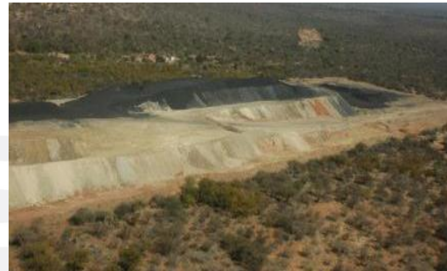
Waste pad with material from bulk sample after processing
