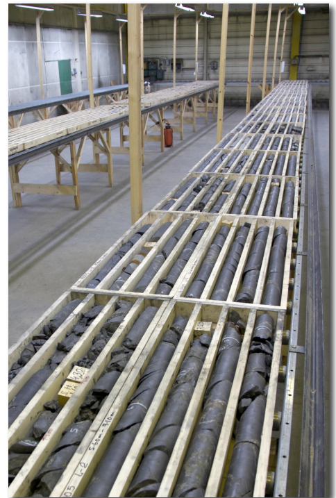
Fig 1. Drillcore from Vittangi graphite project racked up for processing at Kiruna facility.
