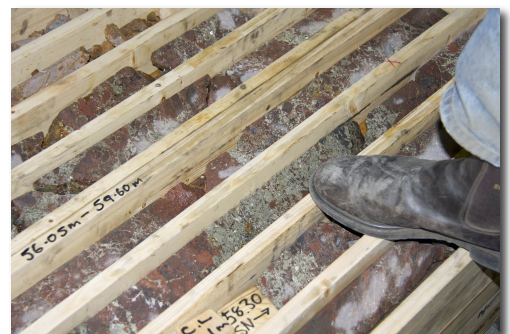
Fig 4. IOCG style mineralisation apparent in Talga drillhole KIS04 (54-58m) Kiskama Project.
