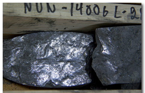
Fig 2. Graphite mineralisation 'slickenside' in drillhole NUN14006, 56m depth Vittangi Project.
