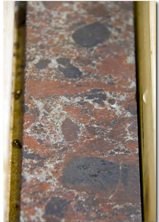
Fig 3. IOCG style mineralisation apparent in Talga drillhole KIS04 (63.1m) Kiskama Project.
