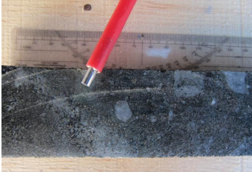
Figure 2: Veinlets of Calcite-Pyrite-Magnetite in intrusive breccia - DDHGI-01. The magnetite is replacing breccia due to intense alteration associated with silicification.
