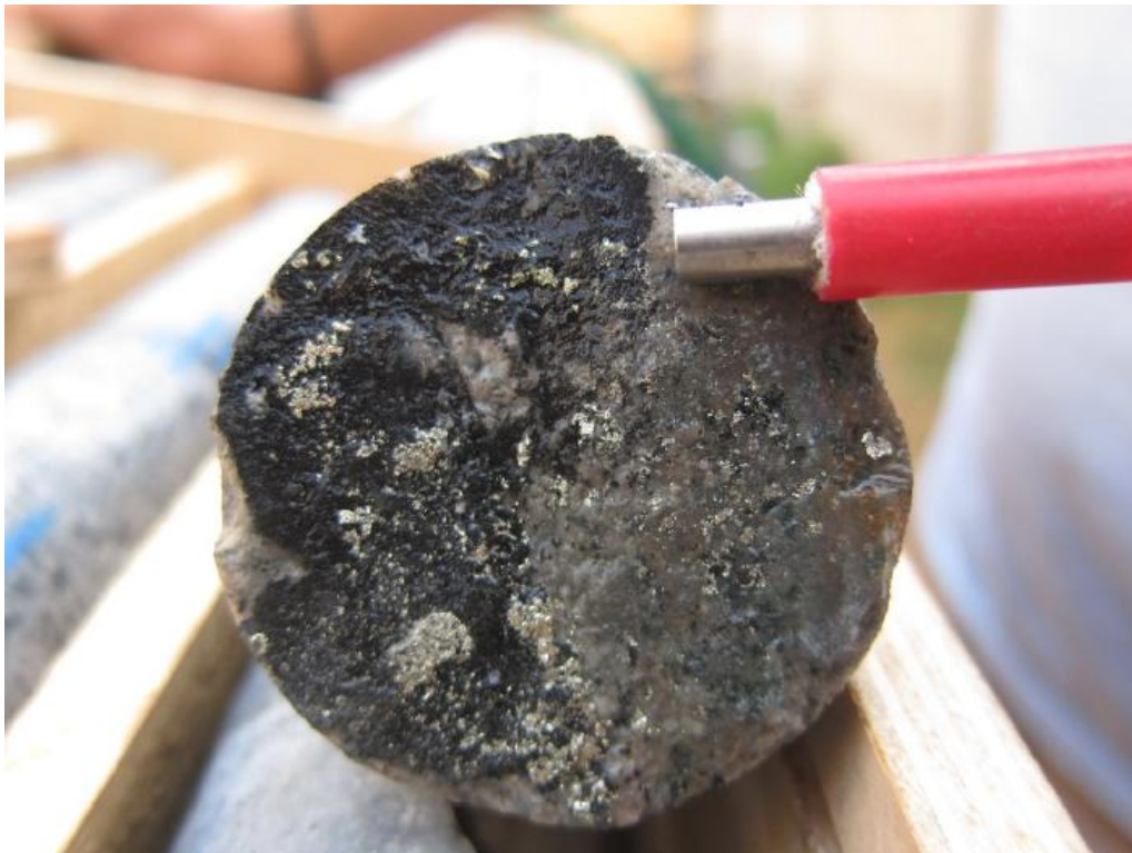
Figure 5: Pyrite-chalcopyrite veins in CMS and tourmaline altered granite, DDHGI-02
