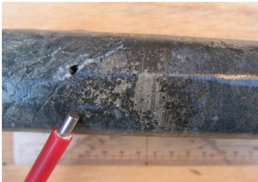
Figure 3: Calcite-Chalcopyrite-Pyrite-Magnetite veining in intrusive breccia, DDHGI-02
