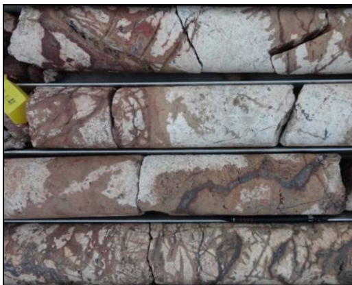
K) Hematite alteration fronts emanating from hematite-filled fractures (S36-001, 20 m)
