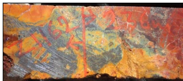
Chalcocite cemented breccia within high-grade supergene zone (S36-038, 236 m)
