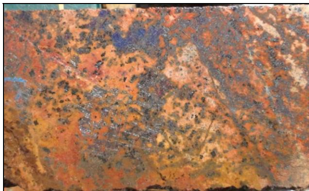
Fracture-hosted + disseminated chalcocite + bornite (S36-038, 236 m)
