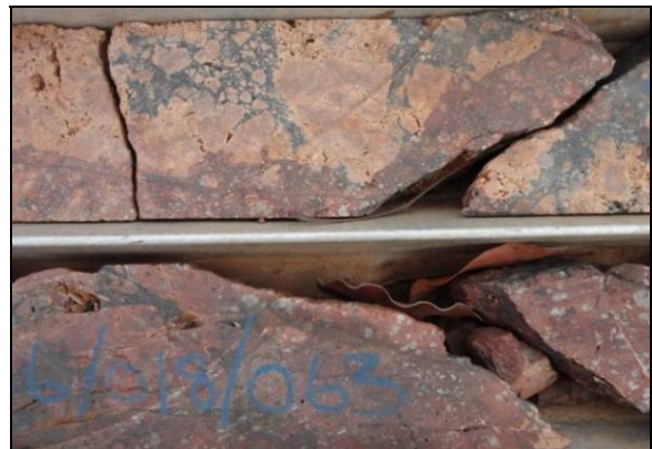
L) Carbonate-matrix breccia clast within iron oxide matrix breccia – evidence for polyphase brecciation (S36-018)
