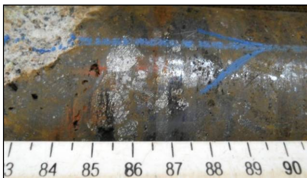
Semi-massive chalcocite in altered syenite within high-grade supergene zone (KITDD_019, 354.35 m)
