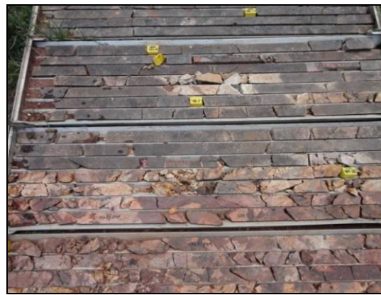
L) Contact between oxidised zone and carbonate alteration (S36-001, 467 m)
