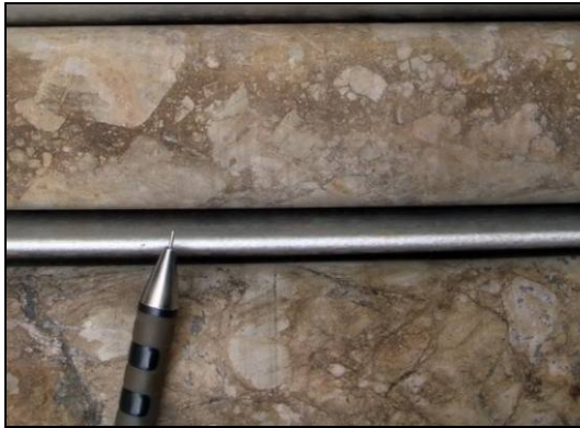
G) Pervasive carbonate replacement of rubble breccia
