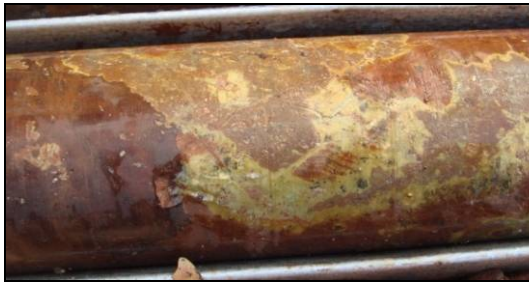
A) Pervasive K-feldspar alteration of syenite (KITDD_009)
