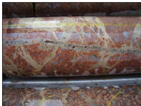
Chalcopyrite-sericite veining in quartz porphyry granite, crosscut by carbonate vein
