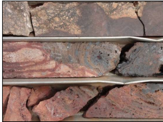
N) Pervasively iron oxide altered metasedimentary breccia clasts (laminated), Carbonate matrix breccia overprinted by iron oxide alteration in the top row (S36-018)
