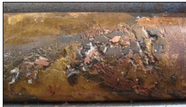
Native copper and calcite in vugs, hematite breccia (S36-015)
