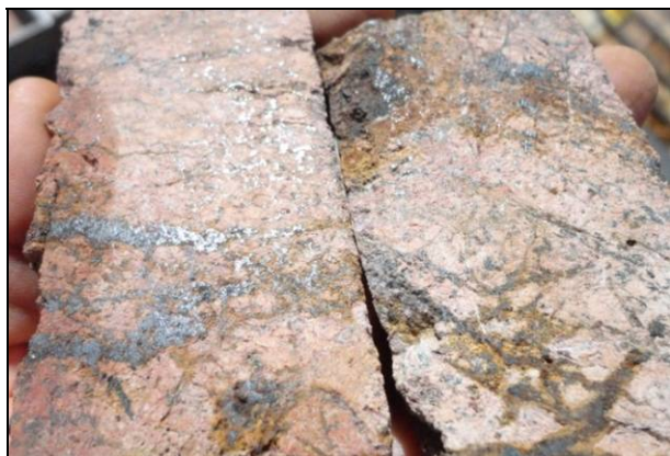
Chalcocite developed mainly along fractures in syenite (S36-033, 222.5 m)
