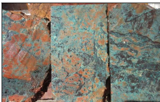
Malachite + pseudomalachite cored by chalcocite \pm pyrite (S36-017 306.2 m)
