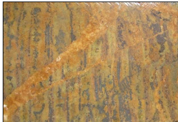
N) Sub-horizontal flow breccia with pervasive carbonate alteration and late siderite veins. Brecciation indicates the proximity to the KFZ (KITDD_005, 603 m)
