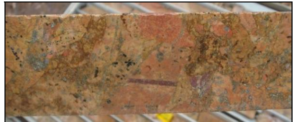
D) Possible polyphase breccia with pyrite mineralisation (S36-017)
