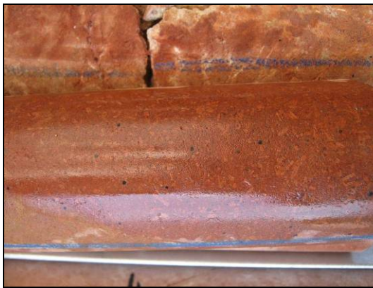
A) Pervasive K-feldspar alteration of syenite (KITDD_009)
