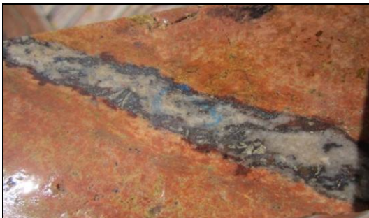
Q) Hematite - quartz vein cutting through K-feldspar and sericite altered syenite (KITDD_009, 483 m). Mineralisation is found only in the hematite vein
