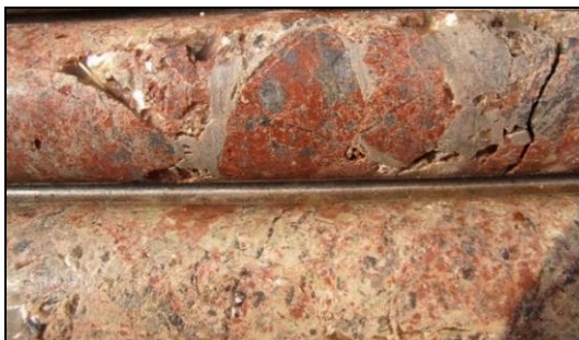
E) K-feldspar alteration overprinted by sericite and subsequently carbonate veining (S3-001)
