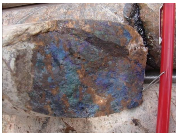
Bornite on fracture surface (S4-001)
