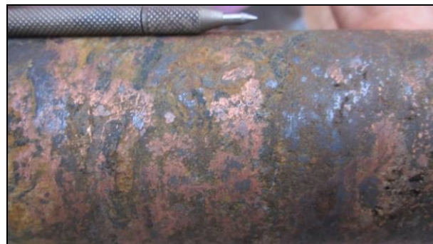
Chalcocite cemented breccia within high-grade supergene zone (S36-038, 236 m)
