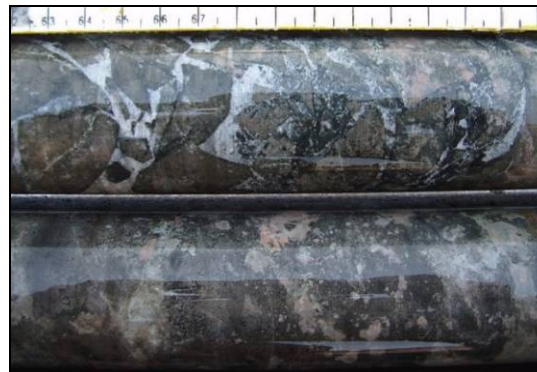
H) Pervasive hematite replacement of metasediments (S36-007)
