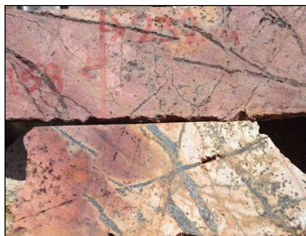
Fracture-hosted chalcocite pyrite in K-feldspar altered syenite (S36-038, 232 m)
