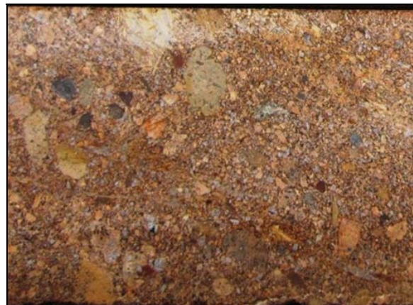
P) Polymictic matrix supported rubble/fluidised breccia with rounded clasts (KITDD_001)
