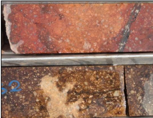
M) Carbonate-altered (bleached by acid) and oxidised quartz porphyry granite (S36-018)
