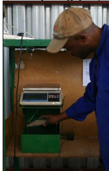
F) Density measurement using a wet-dry scale
