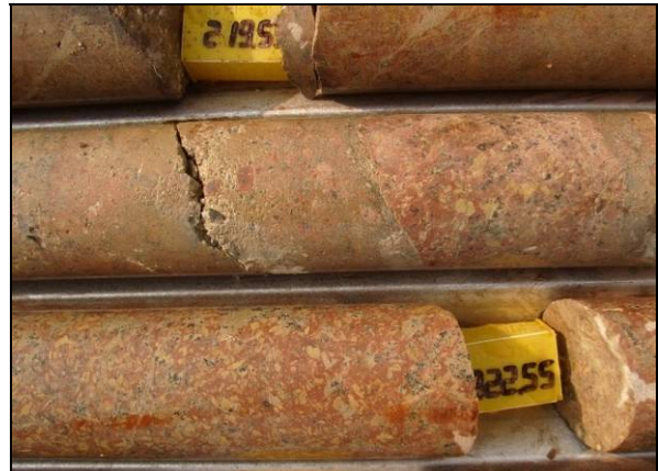
D) Feldspar porphyry diorite/syenite intruding quartz porphyry granite (note xenoliths)
