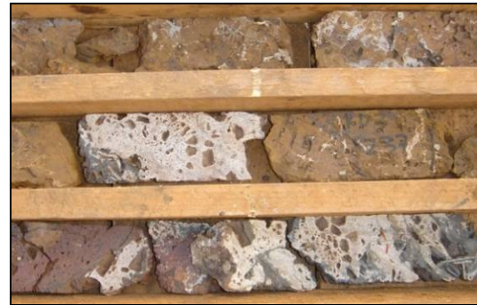
D) Silica alteration overprinting pervasive hematite replacement (KD3)
