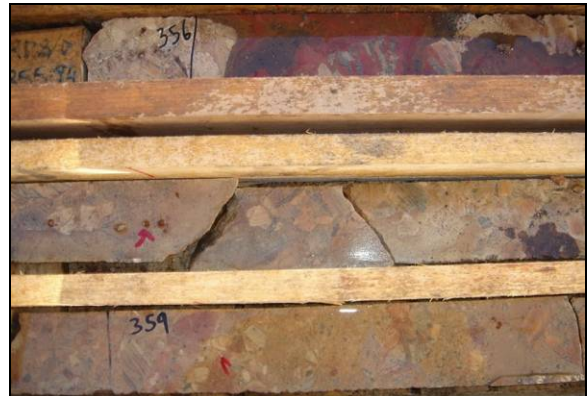
F) Matrix supported breccia in metasediments (KD8)
