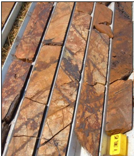
I) Hematite replacement fronts associated with stockwork veining in syenite
