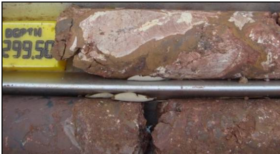
E) Brecciated hematite matrix supported metasediments (S36-015)
