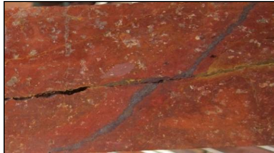
P) Specular hematite vein with a large secondary hematite halo. (KITDD_009, 550 m)
