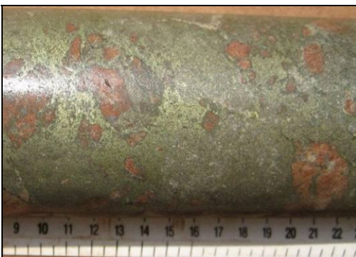
Semi-massive chalcopyrite in altered syenite (KITDD_008, 520 m)
