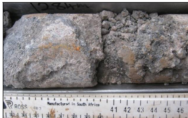
Pyrite and earthy chalcocite vein (KITDD_016, 284 m)
