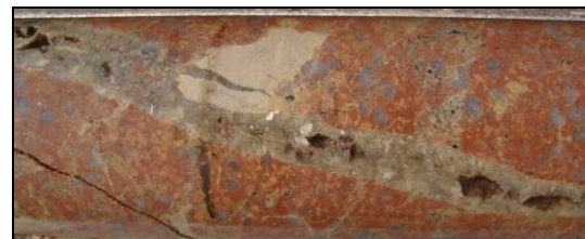
D) Silica alteration overprinting pervasive hematite replacement (KD3)
