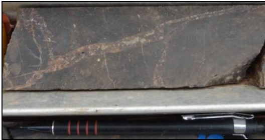
O) Pervasive carbonate altered syenite crosscut by carbonate-pyrite veining (S36-018)
