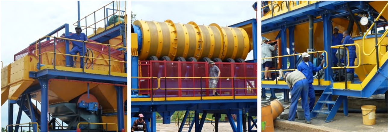
Lucapa's 150 tonne per hour diamond plant at Lulo
