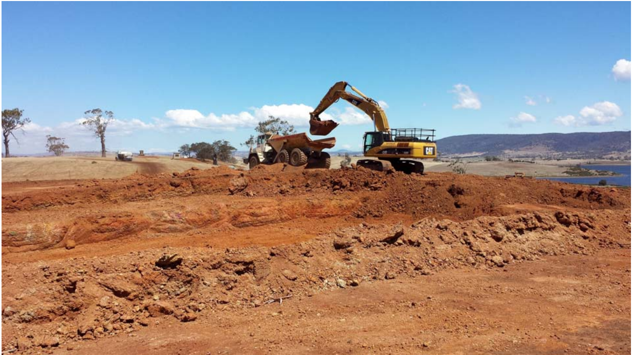
Figure 4: Mining, loading & hauling bauxite ore at Bald Hill Bauxite Project. The bauxite is a surface layer of free-diggable rock up to 6 metres thick. Coarser lumps of bauxite tend to be higher grade and upgrade by screening
