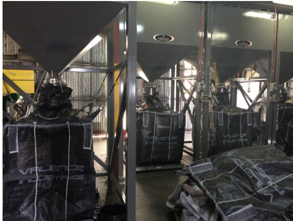
Bagging of Production – 1 tonne Bulka bags
