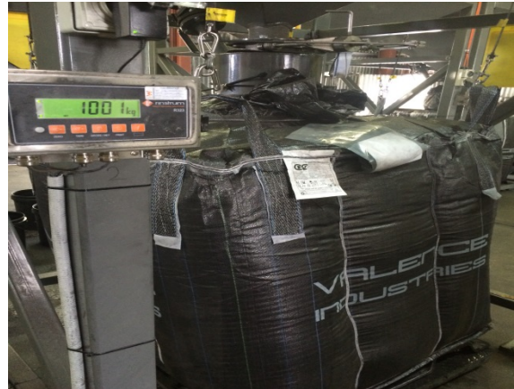
Bagging of Production – 1 tonne Bulka bags
