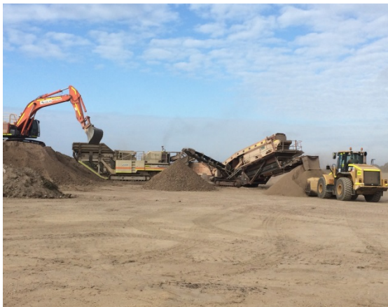
Screening & Resizing of ROM Stockpiles
