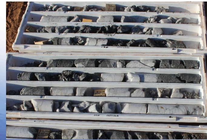
Cross section (above) showing location of diamond drill hole and photo's (right) of quartz veins in oxide zone (top) and primary zone (bottom)
