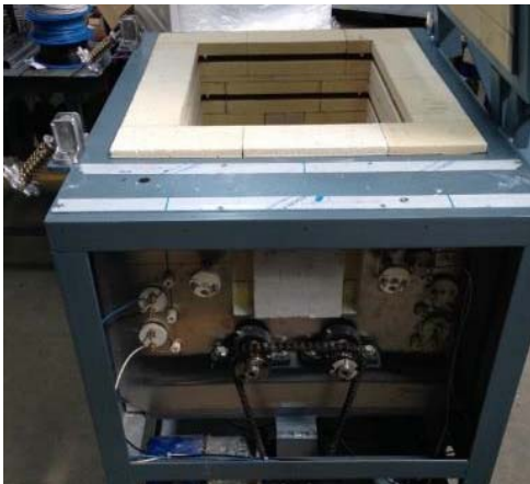
Batch kiln being built
