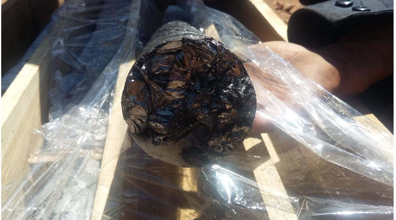
Figure 2- Graphite core recovery from PLB004 showing rosette and needle type graphite with a fragment of quartzite host rock
