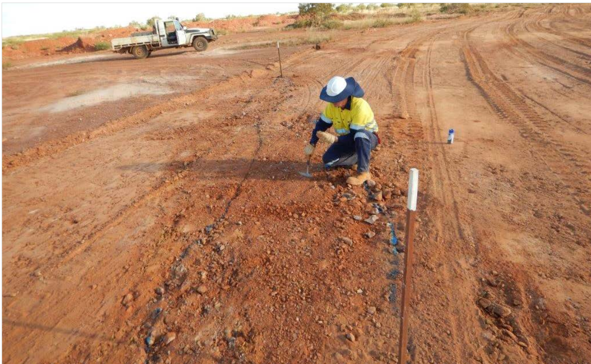
Figure 2. Uncovering never before exposed quartz veins in central zone of Old Pirate (quartz boundaries marked with blue paint lines)
