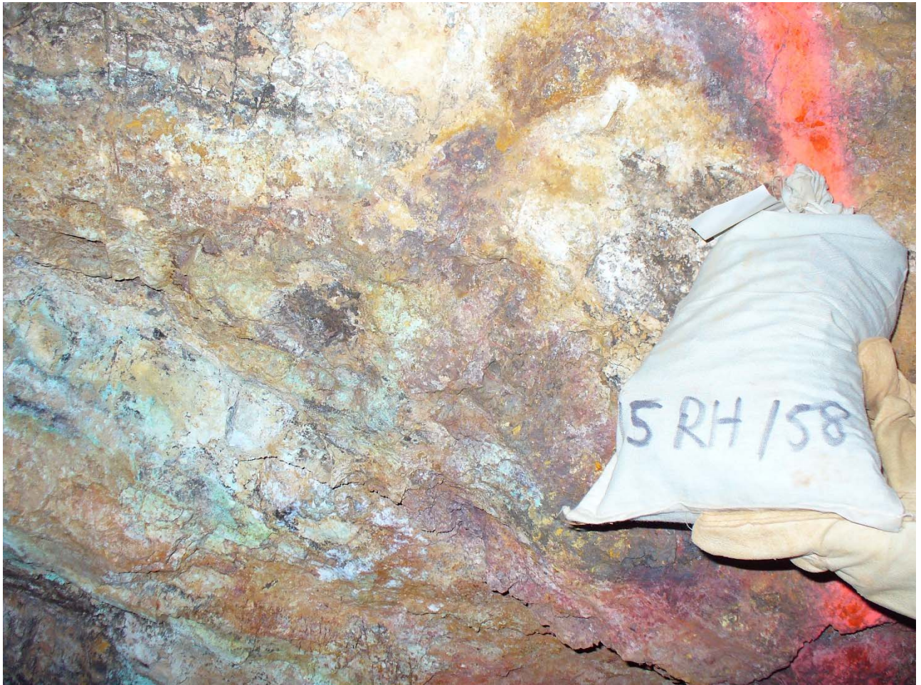
Photo 8 Rattler Thrust Fault – Visible copper mineralisation in breccia (malachite – green mineral in lower portion of photo)
