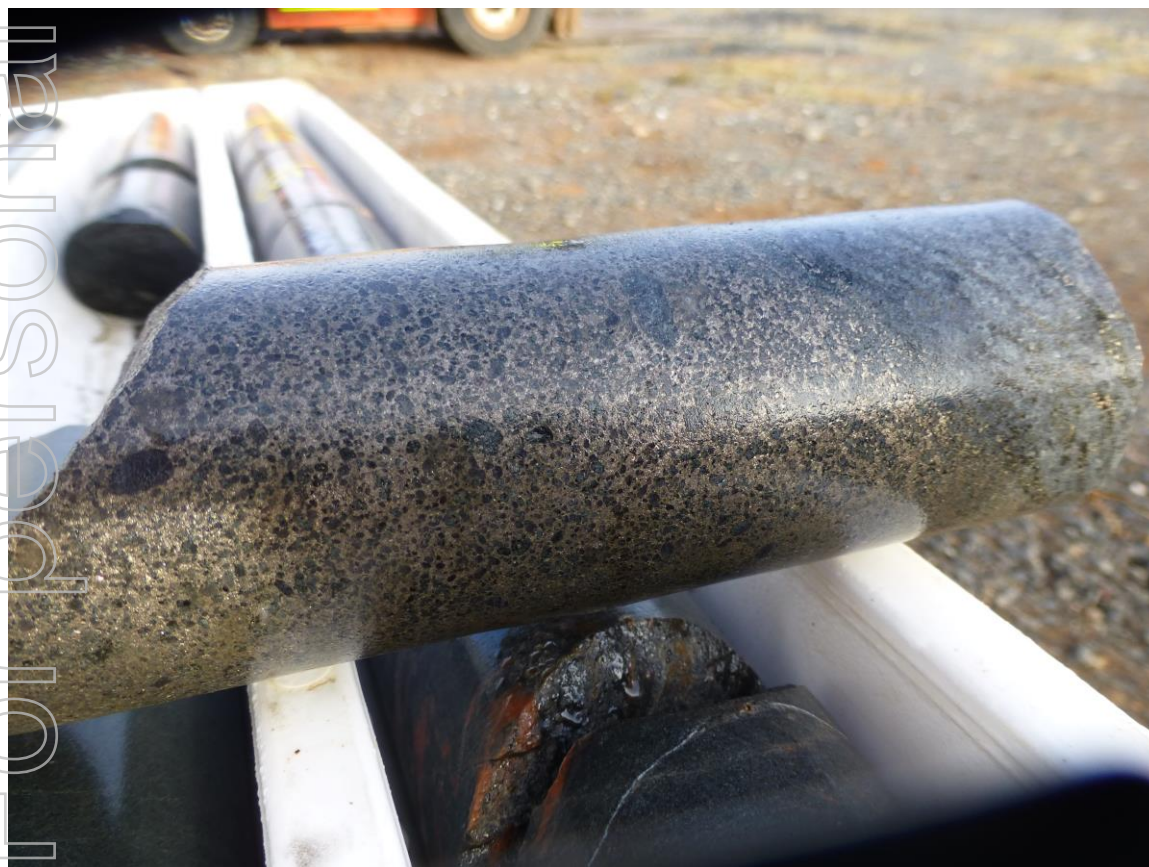
Figure 1: Core at 200m, matrix textured pyrrhotite in an olivine gabbro.
