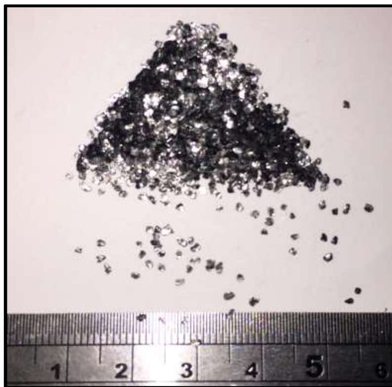
Figure 1 – Extra-large Coarse Flake +35 Mesh Sample from 2015 Uley Graphite Operating Production Commissioning**
