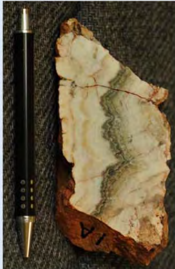
South West Limey Dam Nadia vein (surface) 34.2g/t Gold
