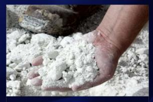
Batch processing included the bulk wet processing of representative samples of future run-of-mine (ROM) kaolin from Meckering to optimise and confirm the beneficiation flow sheet. Beneficiated kaolin was then subjected to HCI processing, which involved calcination; acid leaching to produce aluminium chloride; crystalisation of aluminium chloride; two stages of purification; roasting for acid recovery; and final calcination for the production of finished product HPA.
