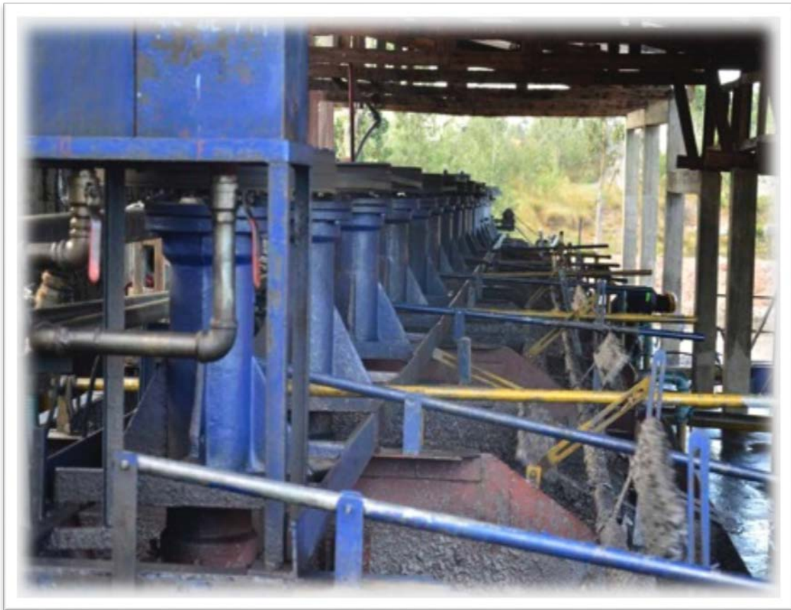
Figure 3: Graphite floatation cells at Loharano
