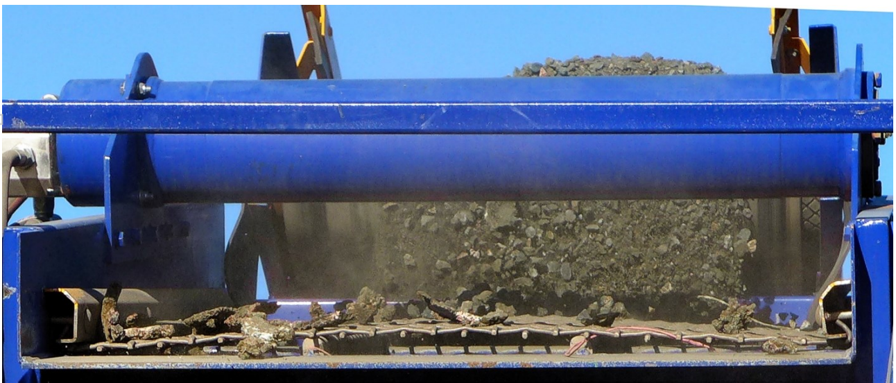
Figure 2: Scalping (recovery) of course native copper by simple crushing and screening. The native copper is flattened during cone-crushing whereas the rock breaks into smaller pieces, facilitating easy removal via appropriate screen sizing.
