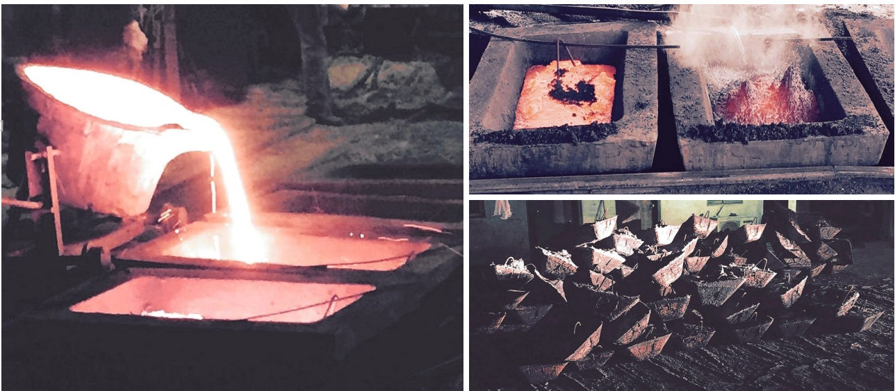
Figure 1: Trial processing of first container of native copper from Rocklands resulted in a final product grade of 99.67% Cu
