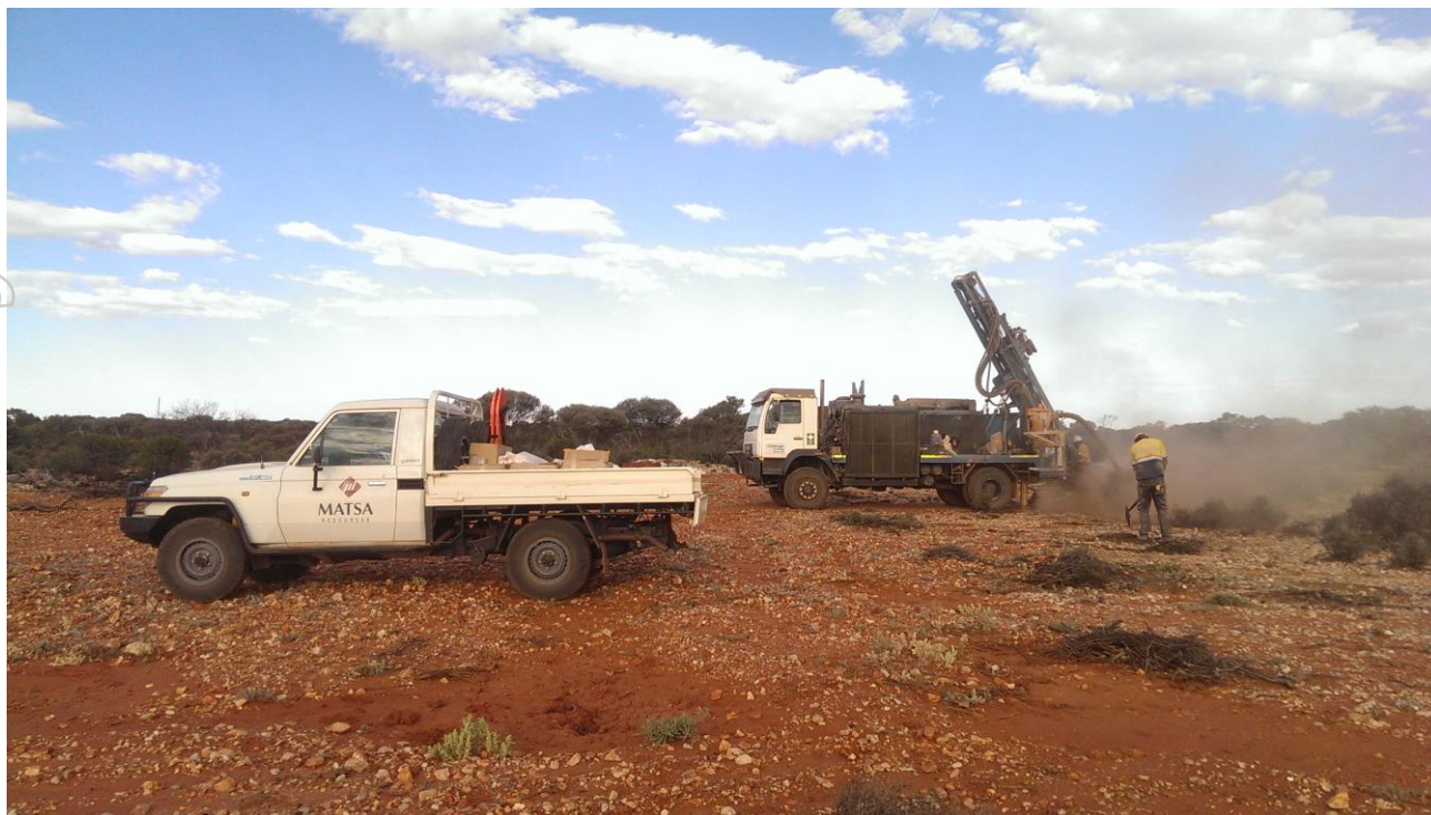
Figure 2: RA150 Aircore drilling rig operating at Point Kidman
