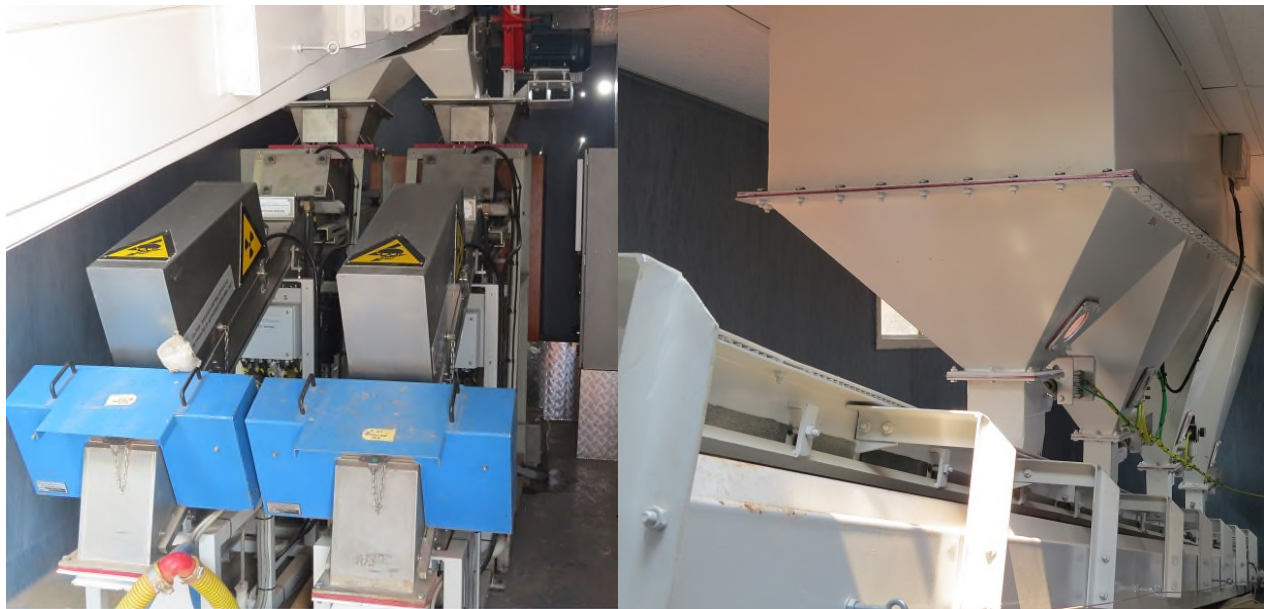
Figure 2: New double pass Flowsort x-ray machines installed at the 150 tph Lulo diamond plant to improve capacity and efficiency of diamond recoveries
