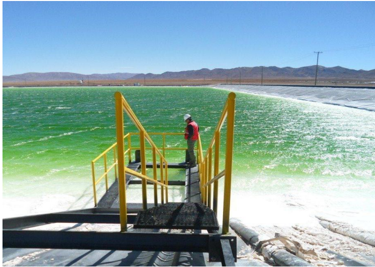
Evaporation pond post magnesium removal/lime addition
