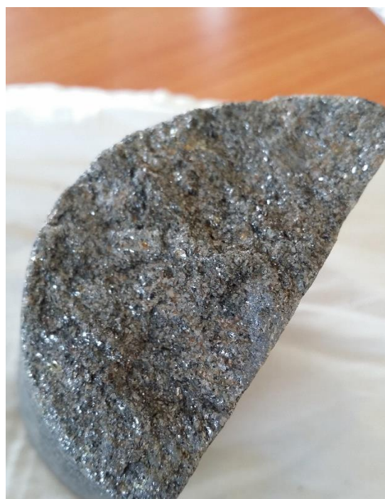
Photo 1: HQ3 drill core (diameter 61.1mm) from holes LJDD002 and LJDD003 highlighting large visible flake sizes.
