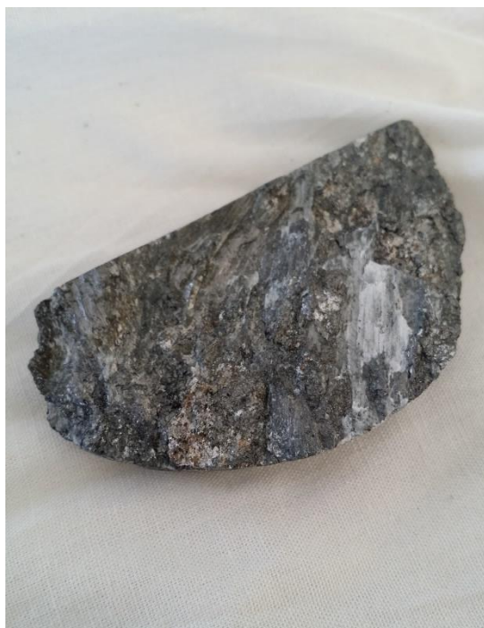
Photo 1: HQ3 drill core (diameter 61.1mm) from holes LJDD002 and LJDD003 highlighting large visible flake sizes.
