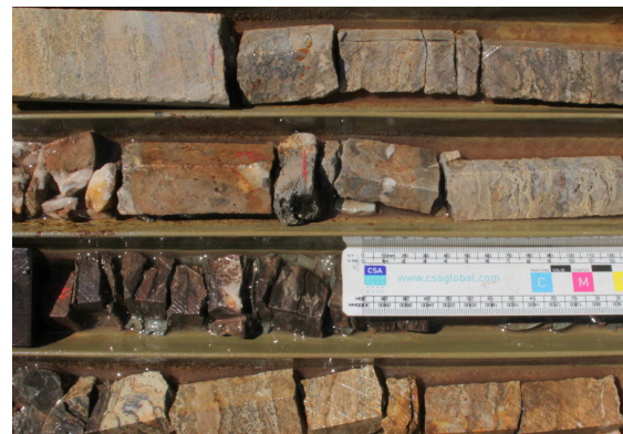
Figure 2. Very high-grade sphalerite (left) & high-grade sphalerite-galena (right) mineralisation
