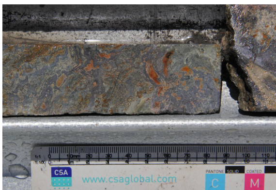
Figure 2. Very high-grade sphalerite (left) & high-grade sphalerite-galena (right) mineralisation
