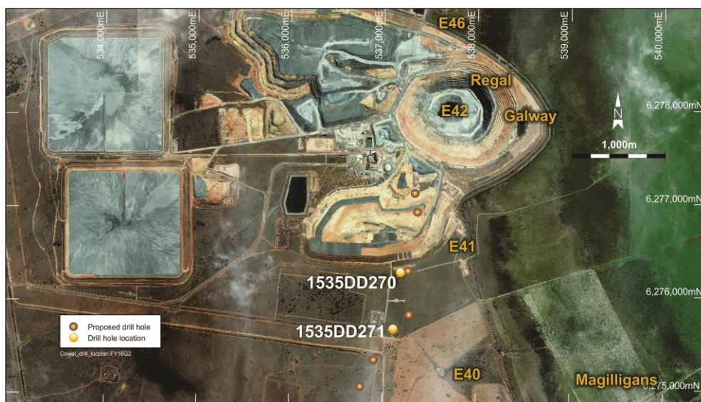
Figure 1: E42 South drilled (labelled) and planned hole collar locations
