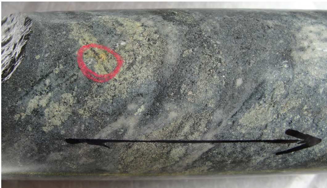
Figure 1. Specks of free gold at the intersection of two fractures in GRDD003. Note association of strong silicification and disseminated pyrite.
