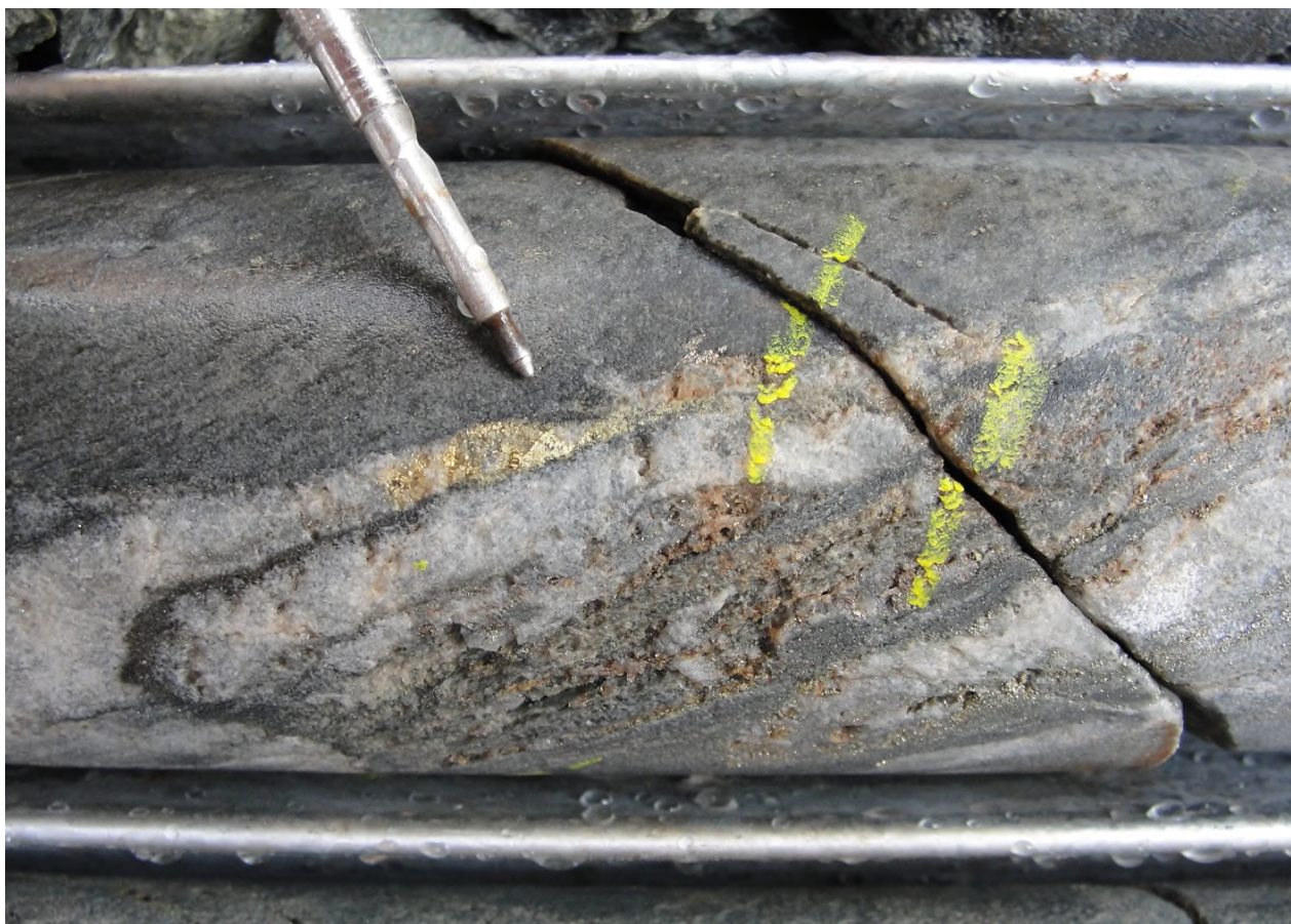
Figure 2. Free gold within a quartz stringer in GRDD007 drilled under the Giro vein.
