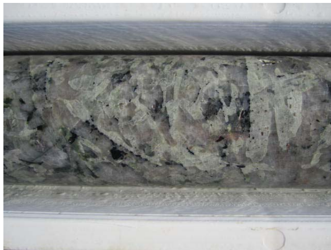
Figure 4: Intense medium-grained spodumene mineralisation in pegmatite from around 177m down hole, below the current resource. Core is HQ diameter (63.5mm).
