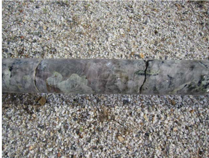
Figure 3: Coarse-grained light-green spodumene crystals in pegmatite from approximately 167m down hole, below the current resource. Core is HQ diameter (63.5mm).
