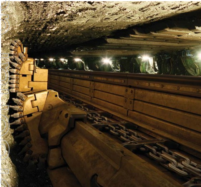
Longwall Plow vs Longwall Shearer face
