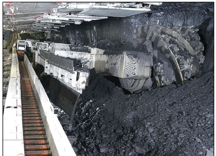
Longwall Plow vs Longwall Shearer face
