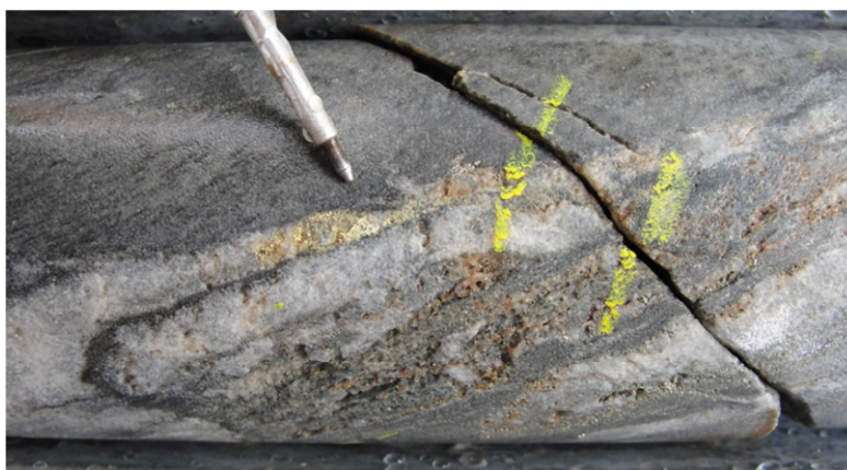
Figure 3. Free gold within a quartz stringer in GRDD007 at the Giro Vein workings.
